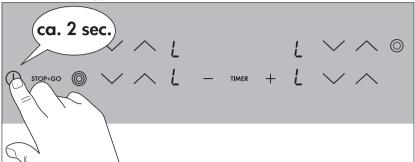
When the child safety device has been activated,  $\Box$  will be displayed. **2.**Touch the stop+go sensor field for approx. three seconds.
